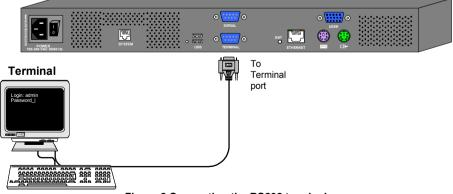
Figure 8 Connecting the RS232 terminal
